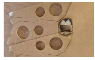
f) Example burn damage at corners during laser cutting, 5mm brown foamboard
