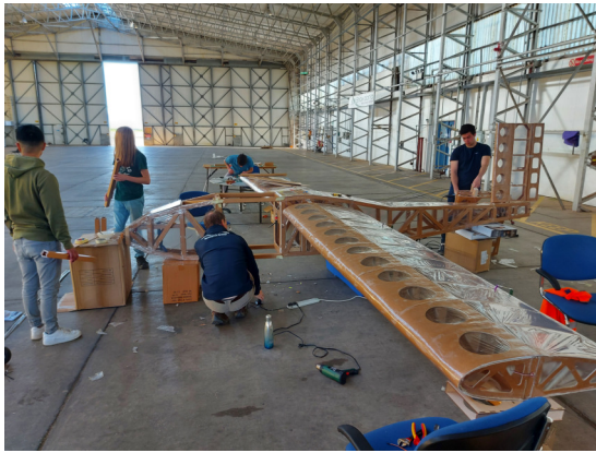
(c) Construction of extended nose structure
